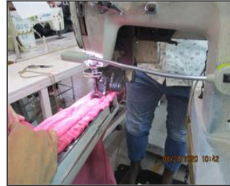
Photo of non-conformity Needle guard were displaced in feed of the arm machine.JPG
