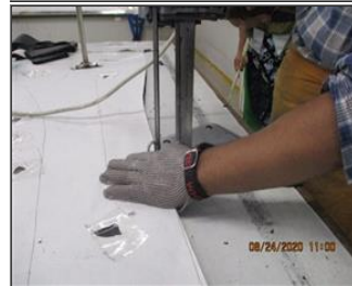
Photo of the personal protection equipments (if applicable) Worker were using metal hand gloves for safety.JPG
