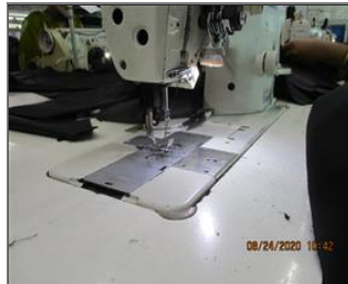
Photo of non-conformity Needle guard was displaced in the sewing machine.JPG
